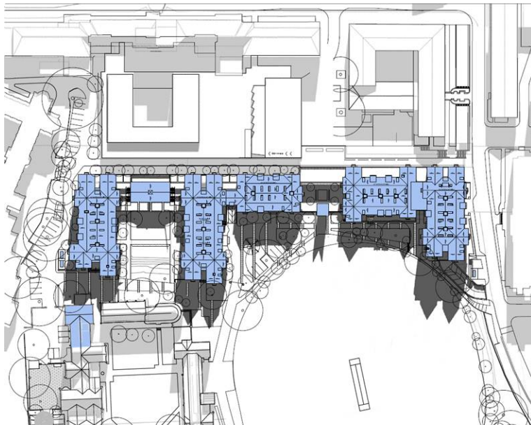
Figure 34: Overshadowing of proposed new buildings onto oval and existing college - 9am 21 June
