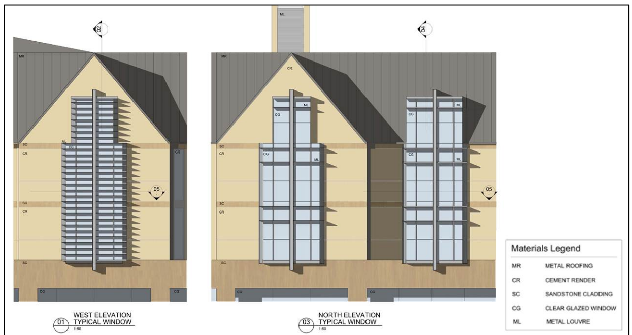
Figure 22: Typical façade and window elevation detail
